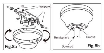
**NOTE:** When installing fan on sloped ceiling, make sure tab on hanger bracket faces towards the top of the slope. Depending on the slope, a longer downrod may be required to prevent fan blades from hitting the ceiling.
